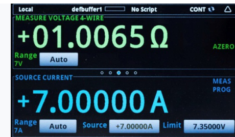
Figure 4. A graphical SMU instrument can display both the source current and four-wire resistance measurement with high accuracy.
